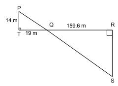
16. This scale diagram shows the measurements a surveyor made to determine the height of a building. What is this height?
